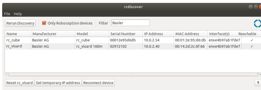
Fig. 4.2: rcdiscover-gui tool for finding connected GigE Vision® devices
